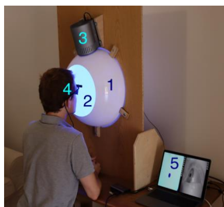
143 Figure 2. Stimulation and measurement system: 1) integrating sphere constructed from two acrylic 144 half-domes, housed and stabilized with a wooden fixing plate, 2) inside coating of Avian-B high 145 reflectance paint to scatter light homogenously, 3) STLAB light source mounted above entry port, 4) 146 Pupil Core eye tracking headset, and 5) laptop running Pupil Capture and custom Python software. 147 The photograph was taken with the participants permission.
